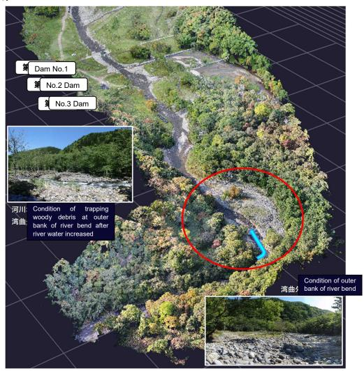
O i Image of trapping woody debris at river flooding
