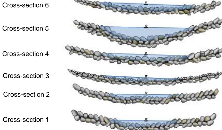
The upper and lower sides of the riverbed channel will be protected by a 50-cm-wide stone riverbed sill. (The cross-section will be arch-shaped to avoid a sharp change in shape.)
