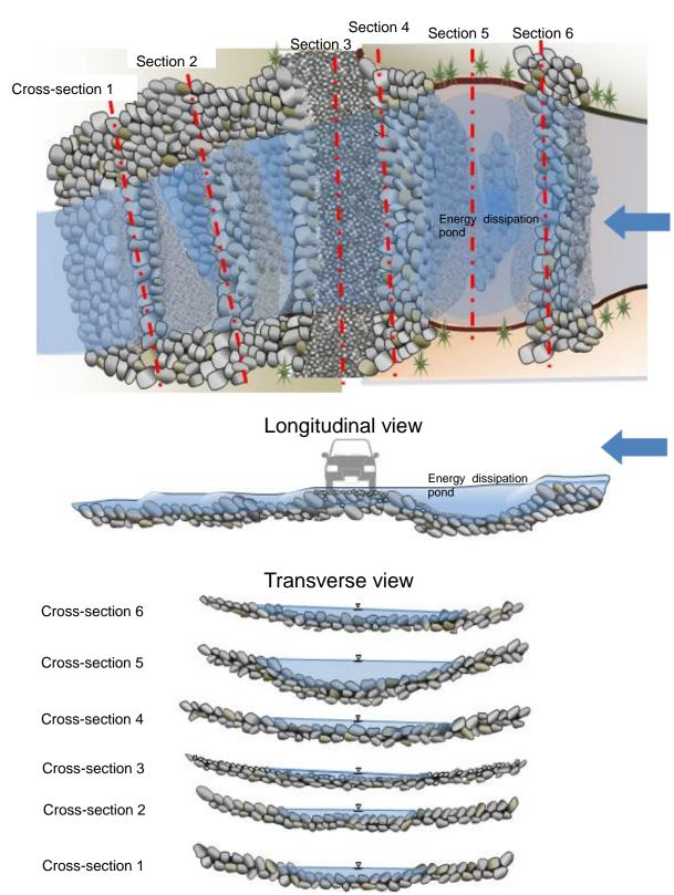
The upper and lower sides of the riverbed channel will be protected by a 50-cm-wide stone riverbed sill. (The cross-section will be arch-shaped to avoid a sharp change in shape.)
